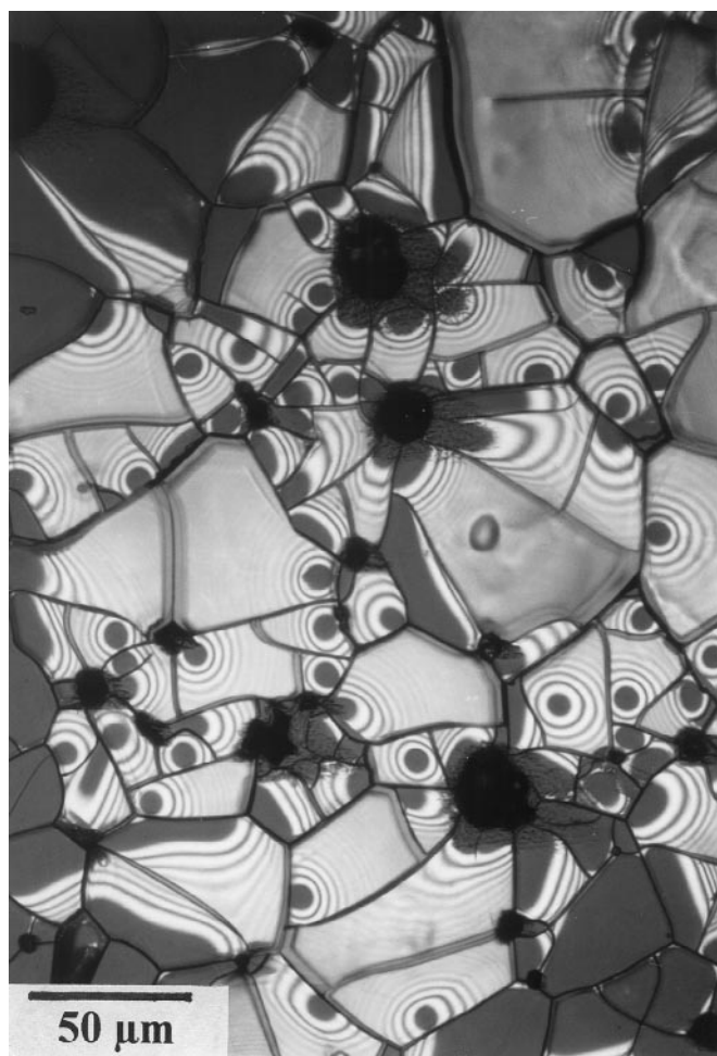
FIG. 3. Optical micrograph of a polycrystalline piece of BCN18 exposed for 2 min at 60°C to a 0.6% HCl solution. (White areas) Here the thick amorphous layer became locally detached from the crystalline matrix due to mechanical coherency stresses as witnessed by the interference fringes arising due to the gap between the two layers. (Dark areas) Here there is still satisfactory bonding between the amorphous overlayer and the crystalline matrix.
